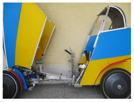
Figure 5 -- Clam door opening for entry/exit
