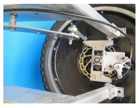
Figure 7 -- Hub, tie rod, and pivot blade beneath swingarm
