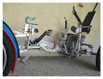
Figure 2 -- Vehicle frame with recumbent seat and arm cranking levers
