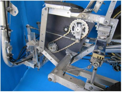
Figure 4 -- Under the seat drivetrain and tilt control elements
