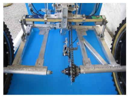
Figure 8 -- Rear swingarms with section of a downhill ski for suspension
