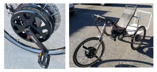
In 2018 Kervelo introduced in-house-built planetary gearboxes with up to 12 gears and a 545% ratio for mounting in front hubs of recumbents and frames of bicycles. Kervelo plan to introduce integrated electric assist for their frame-mounted bicycle gearboxes. Their developments have taken place in parallel, designing fit-for-purpose gearboxes, and simultaneously selling and testing reactions to front wheel drive cycles. Figure 11: Bicycle with Kervelo gearbox, Kervelo Gearbox (Kervelo.com)
