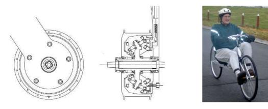
Figure 9: Velotegra gear hub and prototype bike by Jeremy Garnet (Garnet)
