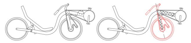
Figure 7: Toxy front wheel drive bicycle.
