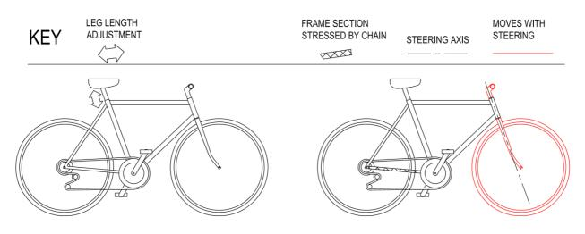
Figure 3: Safety bike and key to diagrams.
