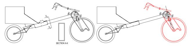
Figure 13: "Murray" front wheel drive bicycle.
