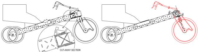
Figure 16: Leaning trike with plywood frame.
