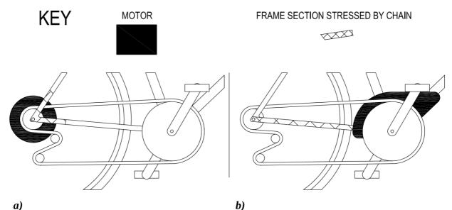
Figure 5: Motors on bicycle a) Hub and b) Crank and how they induce chain stress in cycle frames.
