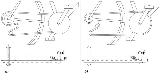
Figure 4: Chain induced stress on bottom bracket a) Low gear and b) High gear. For the same chain tension F1, F2a<F2b.
