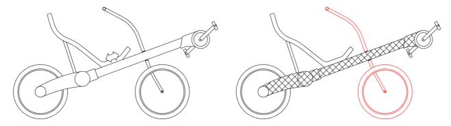
Figure 12: Greenmachine enclosed chain bicycle.
