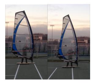
Figure 1. Windsurfer cart under sail pumping power. In the photo at right one can see the sail twists at its aft upper end due to the stroking motion away from the pilot.
