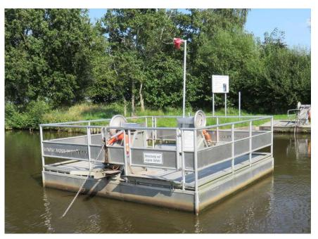
The four self-operated <u>Lippe-Ferries</u> are available seasonally for 2-8 persons. The chains are operated by crankless flywheels, on the ferry or from the shore. In addition, each has a guidance wire, and one of them a longitudinal rope in order to utilize the current.
