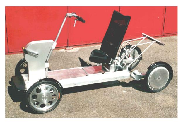
Fig. 2a. Urban Quadracycle, prototype chassis Ultraleicht-Mobiles are related to velomobiles in many ways but are somewhat heavier because fibre plastics are avoided. The vehicle shown was built by Jakob Gilgen from <u>www.gilgen.com</u> (Reference: Bergeron 1999)
